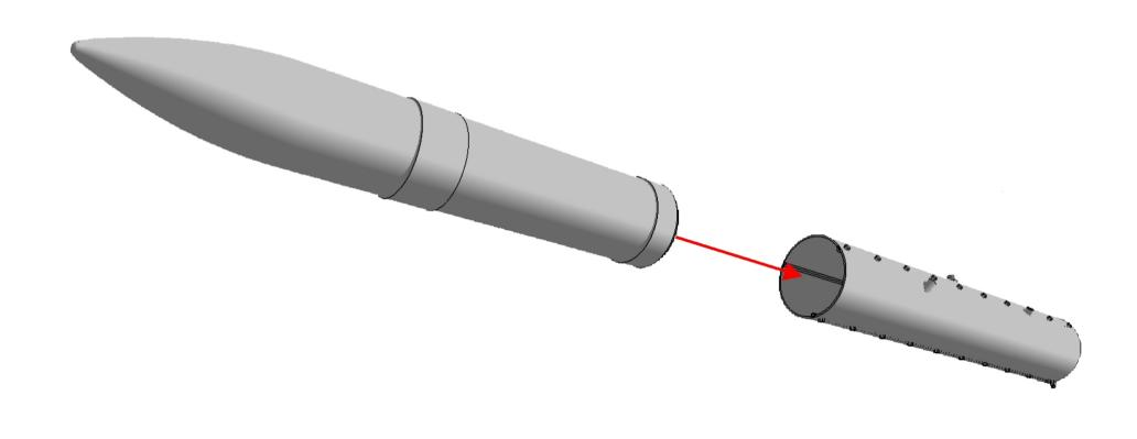
AS SOON AS THE AMMUNITION SHELL IS BUILT, PLACE IT INTO LAUNCHER. ALIGN THE SHELL ONTO THE LAUNCHING TUBE AND SLIDE BACKWARDS (MARKED WITH RED ARROW) CAREFULLY, AS SHOWN ON ABOVE PICTURE. THEN, SECURE IN PLACE BY ADDING A DROP OF CYANOACRYLATE SUPER GLUE.
