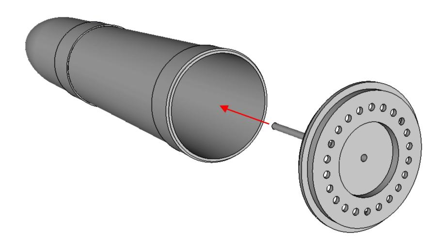
INSERT THE DISC SHAPED REAR CAP AND CLOSE THE HOLLOWED AMMUNITION SHELL AS SHOWN ON ABOVE PICTURE. USE EXTRA CAUTION WHILE INSTALLING REAR COVER & AVOID VIOLENT MOVES TO PREVENT PLASTIC FRACTURE & SECURE IN PLACE BY ADDING A CYANOACRYLATE SUPERGLUE DROP.
