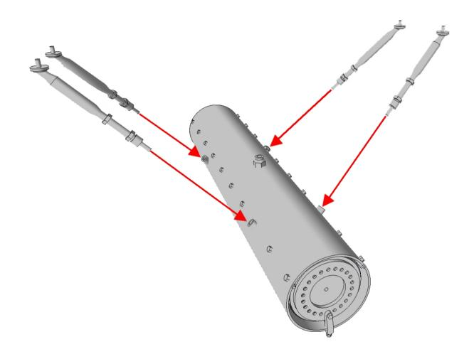
THE KIT CONTAINS TWO PAIRS OF DIFFERENT LENGTHED CYLINDRICAL SHAPED SUPPORTING BARS.
