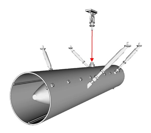
THE KIT CONTAINS ONE CENTRAL BOLT EQUIPED WITH HOOK, WHICH IS THE MAIN UNDERWING SUSPENSION POINT. HOOK'S BEAM HEAD SHOULD BE ALIGNED ONTO BOLT'S SLOT (MARKED WITH RED ARROW). AVOID VIOLENT MOVES WHILE INSTALLING THE HOOK ON BOLT TO PREVENT DAMAGE.
