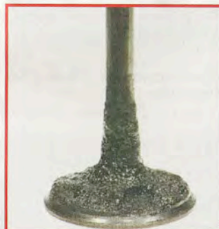
Intake valve before PI. treatment
