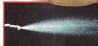
Injector spray pattern after PI. treatment
