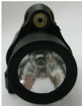
IMPOSTER: Bumpy coating for reflector. Brass laser aperture
