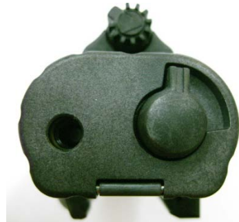
INSIGHT: Remote Jack is typical Insight – 2 outer rings – no pin in middle.
