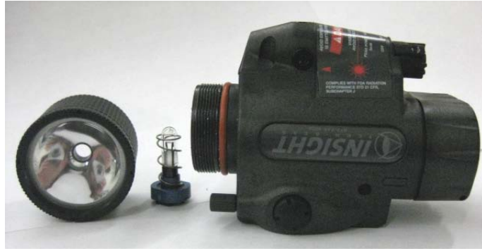
INSIGHT: Bezel and reflector in one. Spring around bulb
