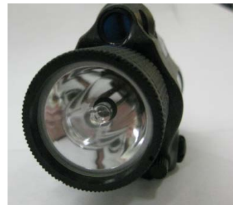
INSIGHT: Smooth shiny coat for reflector. Dark metal laser aperture.
