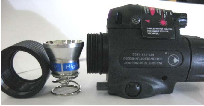
IMPOSTER: Bezel and reflector are separate. Spring on end of reflector.
