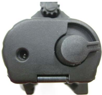
IMPOSTER: Remote Jack looks like a DC adapter jack with pin in the middle
