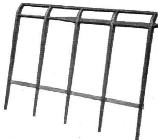
View showing a portion of the skeleton framework of the elevator on the Macfie monoplaner.
