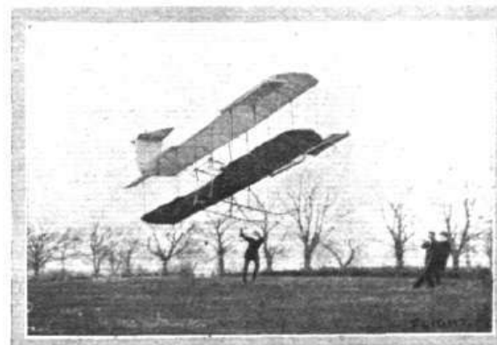
The "Mayfly" in its original form as a glider, soaring in a 12-m.p.h. breeze.
