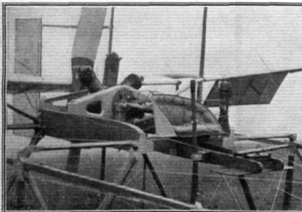
Detail views of the Valkyrie monoplane racer, showing (on the left) the pilot's seat and mounting of the Gnome engine. The right-hand view shows the two small "prows" under the fixed front plane.
