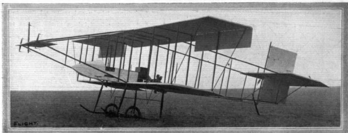
Side view of the latest Short biplane, showing the enclosed car for the pilot and passenger. The horizontal rib in the extremities of the main planes, which are cambered elsewhere, is a curious feature of interest.
