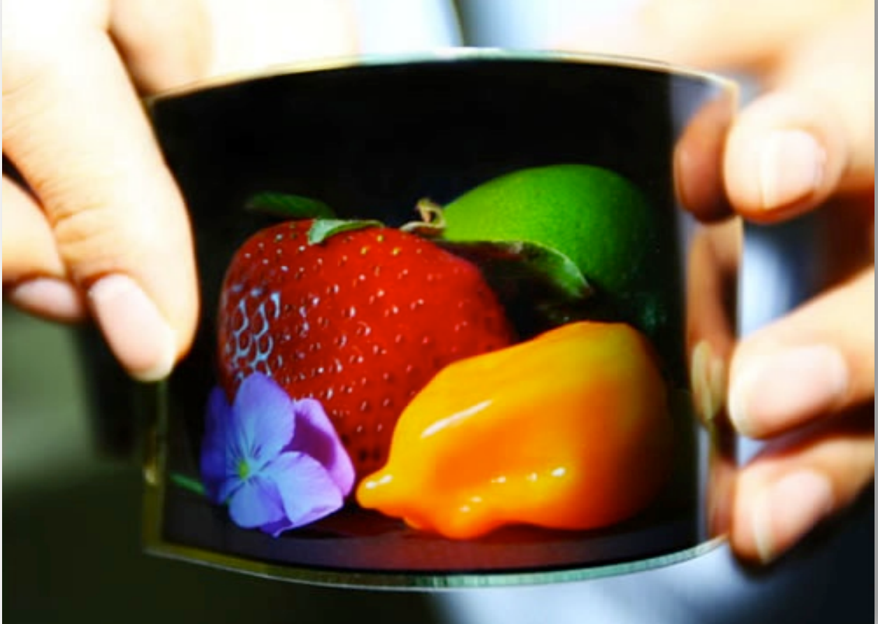
Figure 8: Samsung flexible AMOLED 4.5 inch 800 x 480 display only 2 mm thick (a) at CES 2011 and (b) at FDP-International 2010
