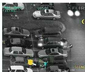
Low-light TV camera provides clear visible-light imagery in near total darkness.
