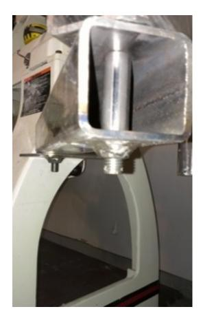
Next I drilled a 3/8" hole 1 1/2" down from the top edge of the T head for the bar locking lever. I then proceeded to weld a 3/8"-16tpi nut to it in the same manner as above. Adding a second hole and nut to one of the other sides may come in handy for possitioning of the lock lever on larger turnings.
