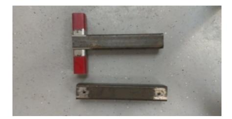
Next I drilled a 1/2" hole through the top and bottom of the oposite end, and through the top and bottom of both ends on the second arm. These hole were located in the center of the 2 1/2" tube at a distance of 1 1/4" from the ends. The holes were step drilled, starting with a 1/4" bit and working my way up to the 1/2" bit.
