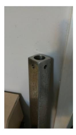
Instead of going back and chancing messing everything else up here, I'm showing the black pipe sleeves below. These sleeves go into the square pipes so that the 1/2" bolts pass through them. Having these in place will add stiffness to the square pipes when the bolts are tightened down, lessening the chance of deflection in the pipes. You need to make 3 of them.
