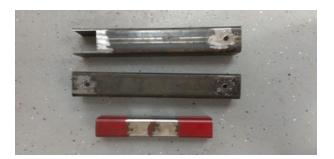
After all parts were cut to length, I started with the arm that accepts the T head. I used my jig saw with a bi-metal blade for cutting a notch out of it 2" wide and 2" deep. The top and bottom are cut out leaving the sides for support and more welding area. This could also be done a number of other ways.
