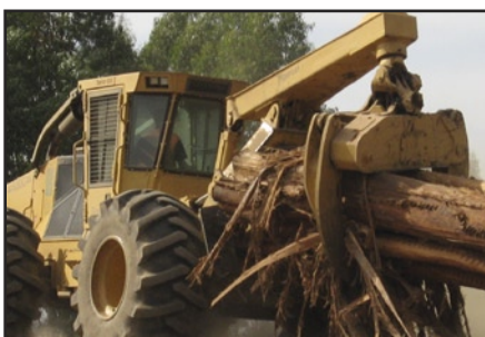
Clear line of site to rear tires, grapple and arch; high capacity Tigercat grapples
