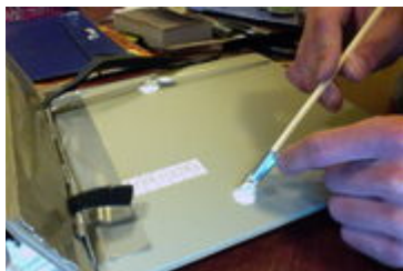
Figure 22: Fastening skewers to back of front panel.
