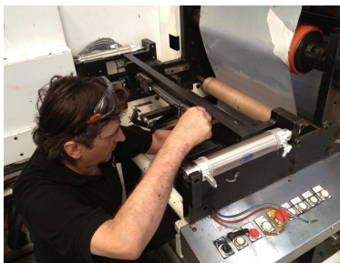
Above: Serge De Jardin of ETI Canada installing the new Labeline adhesive coating head.
