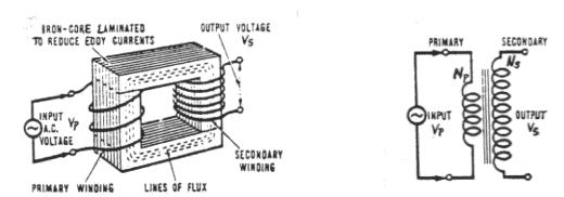
The size of the secondary voltage compared to the voltage applied to the primary depends on turns ratio, or transformation ratio. That is, the number of turns of wire in the secondary winding compared to number of turns in the primary.
