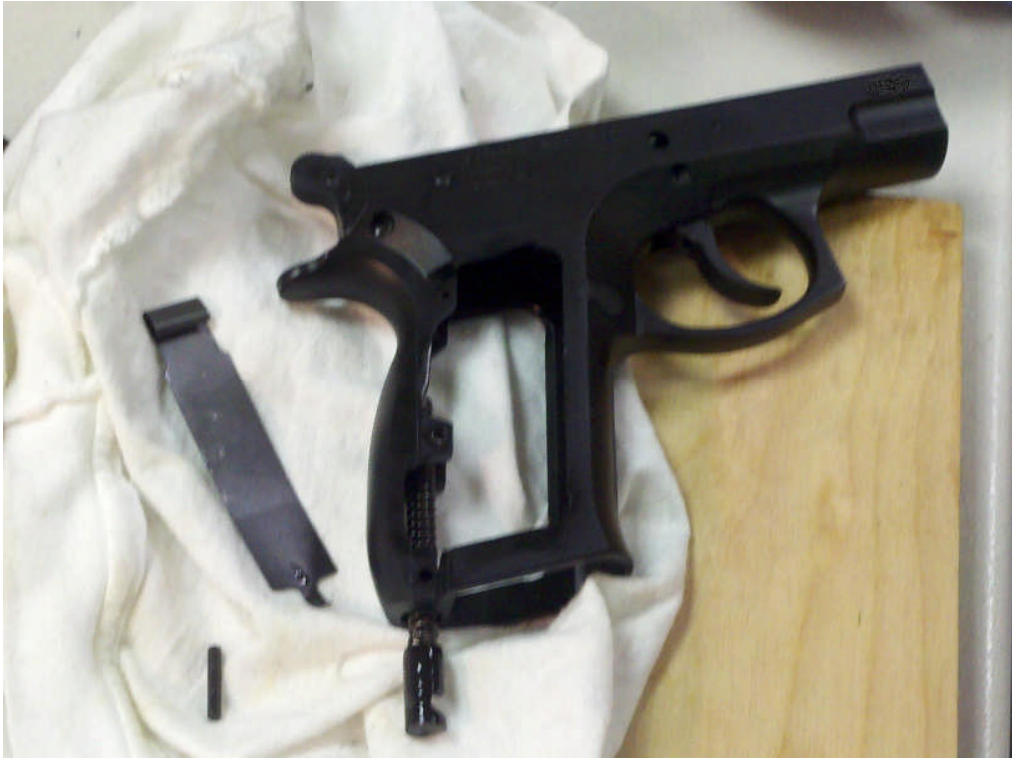
Mainspring plunger/plug, magazine brake, mainspring, and pin is now out
