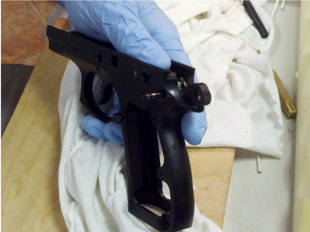
Here is the hammer pin coming out
