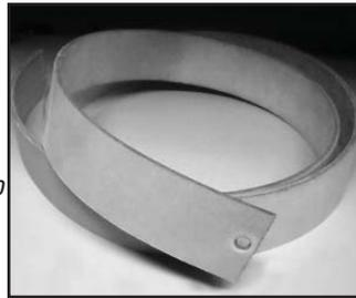
Use a good quality leather contact cement like Tanners or barge. When you connect the two pieces together, use a hammer to pound the finished side smooth. Run the belt in the direction that won't peel back the joint. Mark that direction with a marker on the inside of the belt. Keep the speed down so it doesn't fly apart. Use with Flitz, Green Chrome buff or other very light abrasive compound.
