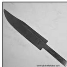
Hand-forged, 1085 high carbon steel by Windlass Steelcrafts®. Tempered to approximately 50 R.C. The narrow fuller runs 1/2 the length of the blade.
