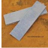
This material is polyester resin reinforced with polyester textile; whereas g10 and micarta are made with a phenolic resin. The polyester resin makes for a more stable handle material that will not crack or break and has negligible water swell. This material is best for tactical knives that require a handle with no slip.
