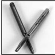
These are tapered taps that push the chips ahead of the cutting to keep the flutes clear and free from jamming up.
