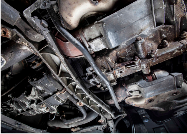
Clockwise from left: Exhaust heat shield missing, underside shows use, build-up of grime on gearbox
