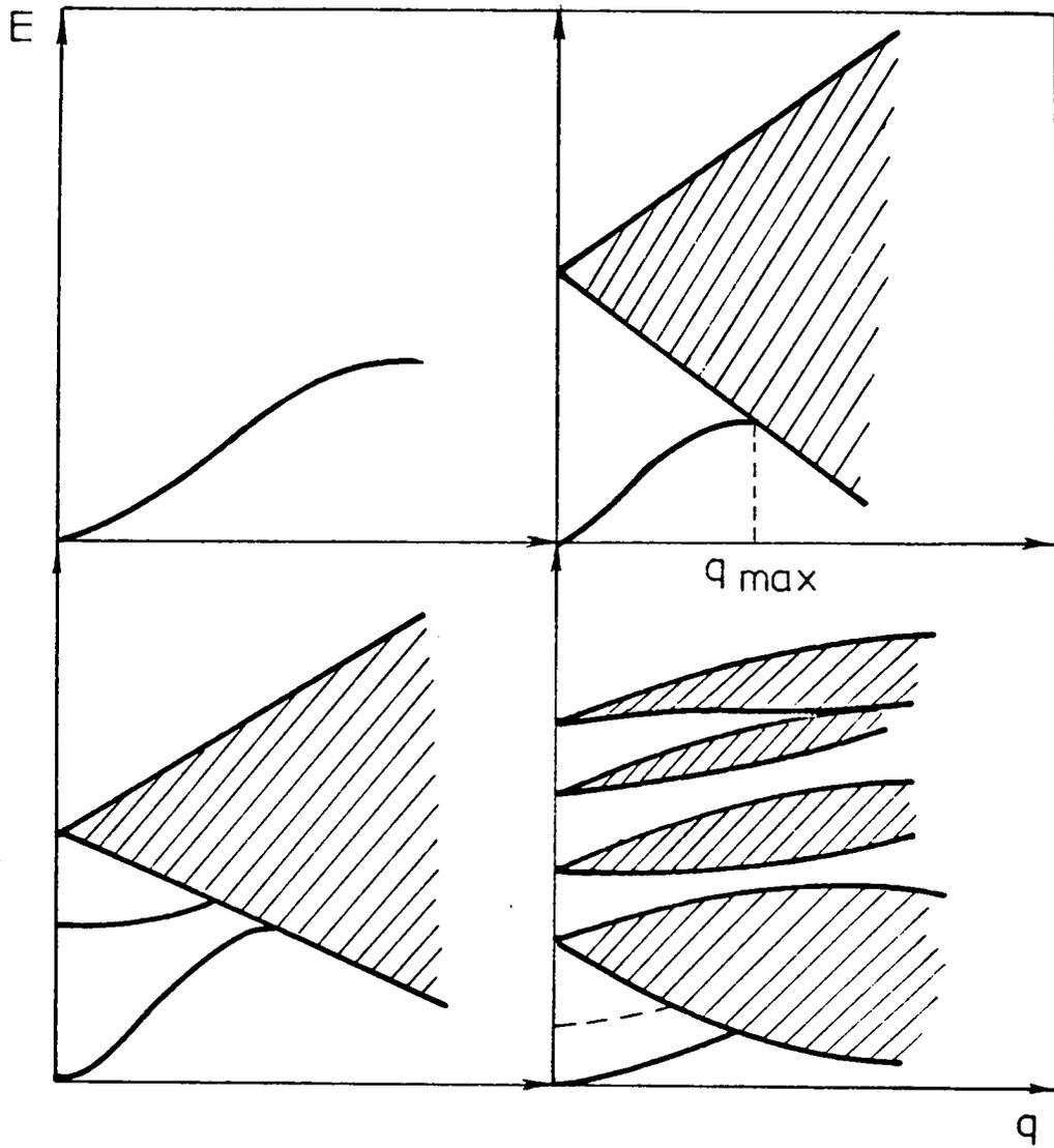
Figure 1: Schematic form of the excitation spectra of the four microscopic models of magnetism: a) upper-left, the Heisenberg model; b) upper-right, the Hubbard model; c) down-left, the modified Zener (spin-fermion) model; d) down-right, the multiband Hubbard model.
