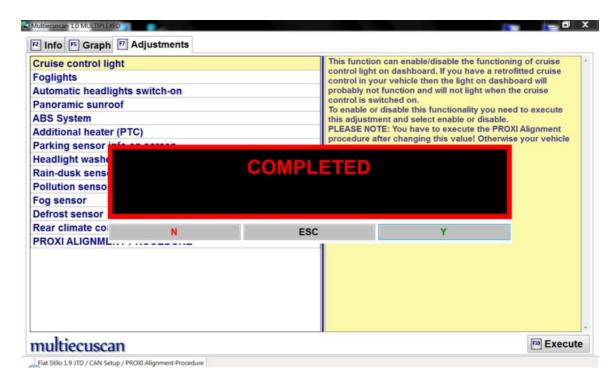
**Step 8:** Now we have to execute the PROXI Alignment procedure to write the new settings to the car.
