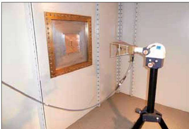
FIGURE 5: Test set-up in receiving room
