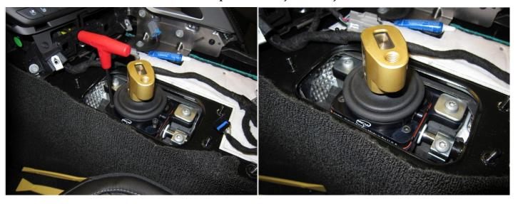
Use the included Allen wrench to tighten the locking set screws (4 in total).
