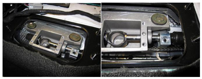
Carefully, using a steel panel tool or similar, 'pry' the factory box upward using a gentle twisting motion:
