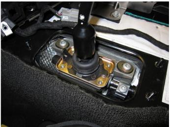
Use a screwdriver or other rigid tool to 'pry' locking pin upward:
