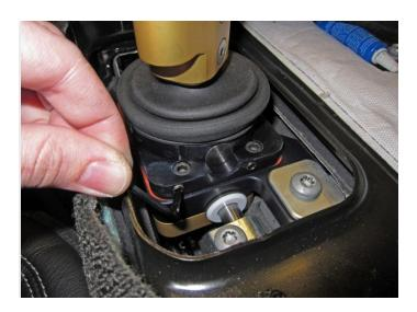
In order to make room for the MGW rubber boot, the stock cover will need to be slightly modified. This cover is bit different from the C6, but essentially the same. You will make the exact same cut as seen here:
