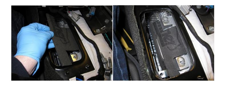
Prepare the lower box w/ grease (sparingly), and make sure to move the rod back and forth to work it in. Do not add so much that it becomes more difficult to move the rod!
