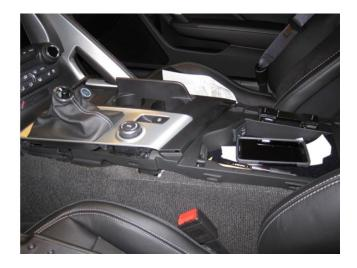
Continue removing the top panel by releasing remaining clips with a panel tool. Slowly lift up and away from the dash to release the two front curved sections.
