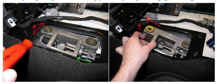
Slide the lower box out carefully, keeping in mind to separate the rod from the clamp.
