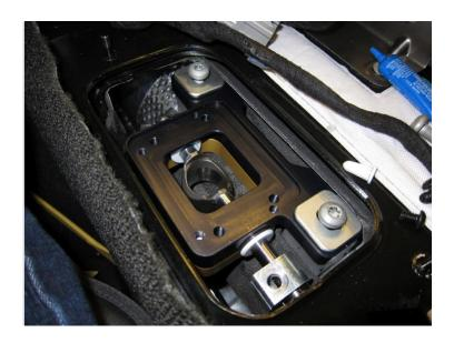
The alignment tool included works very well - leave the four screws loose until you eyeball the notch. Once it's dead on, crank those screws down.
