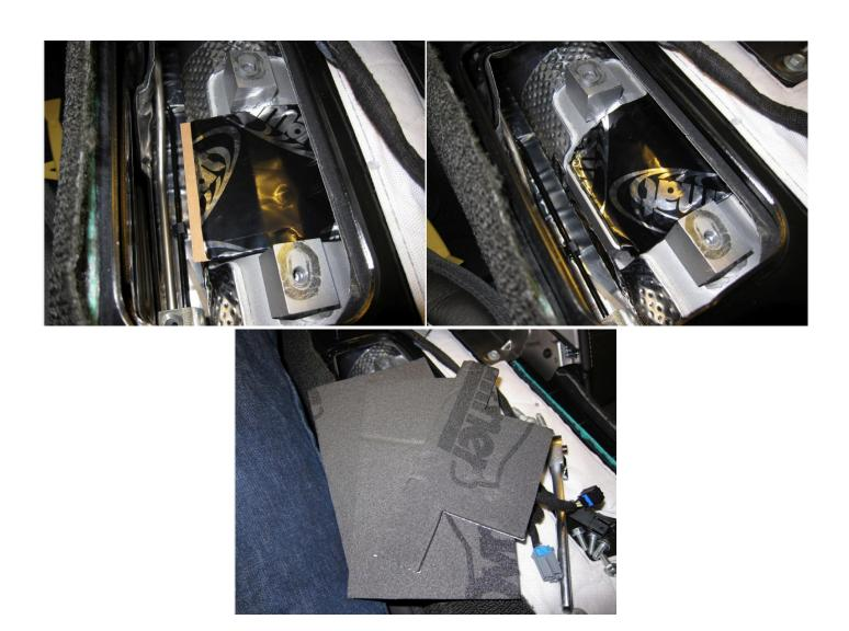
This part is notoriously annoying. Peel back a small amount of the backing before shoving the piece under the torque tube:
