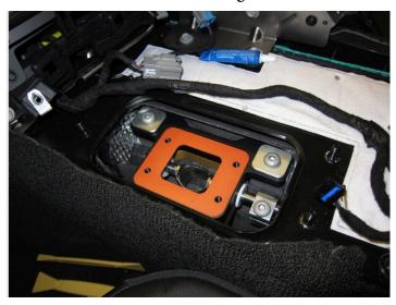
Install the shifter with the text facing the driver:
