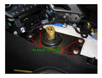
Align and tighten the shift knob shaft (with nut, locking nut, and washer as shown). Use the stock knob to eyeball/align the screw hole. For the C7, it should be dead center left-to-right.
