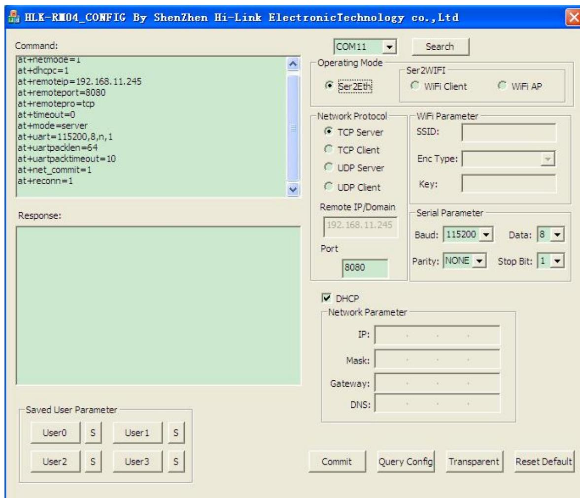
Chart 17 Serial configuration tool generates AT command
