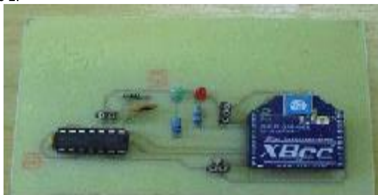
Figure: 2.2. Fabricated sensing unit with ZigBee module.
