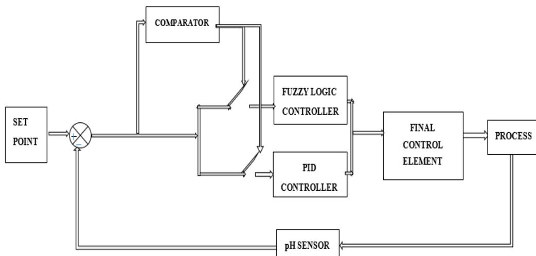
Figure.1. Block diagram of the process with controllers choosing either PID or fuzzy controller
