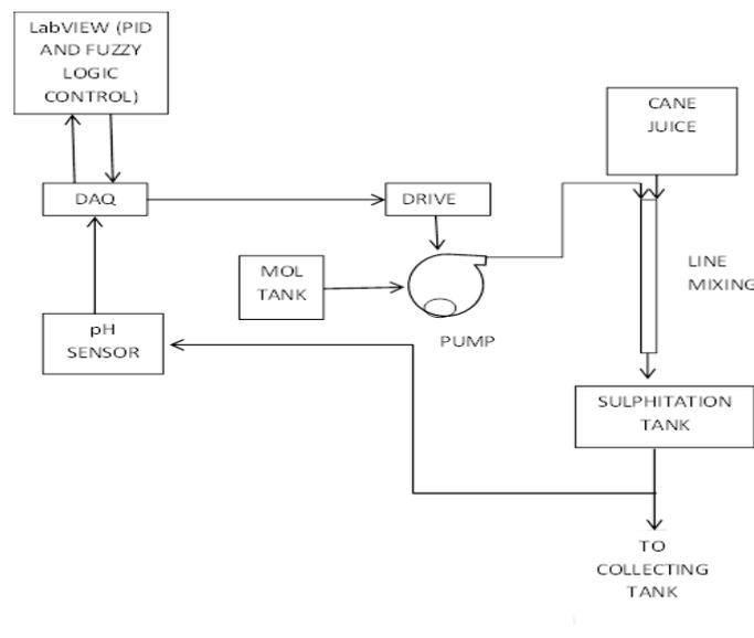
**Figure.2.**Block diagram of the proposed model of pH automation in the sugar manufacturing unit
