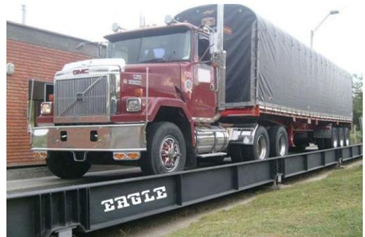
In [Pitless Type Weighbridge](#) RCC ramp work must be required at least 3 meters for both sides for easy movement of vehicle.
