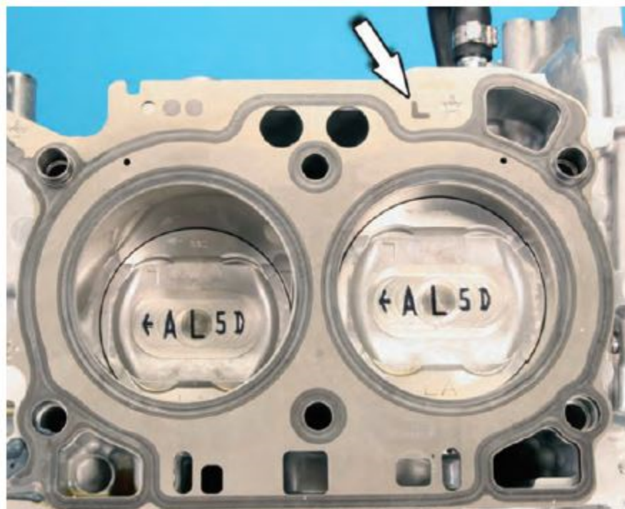
Head gaskets are marked “L” and “R”.
