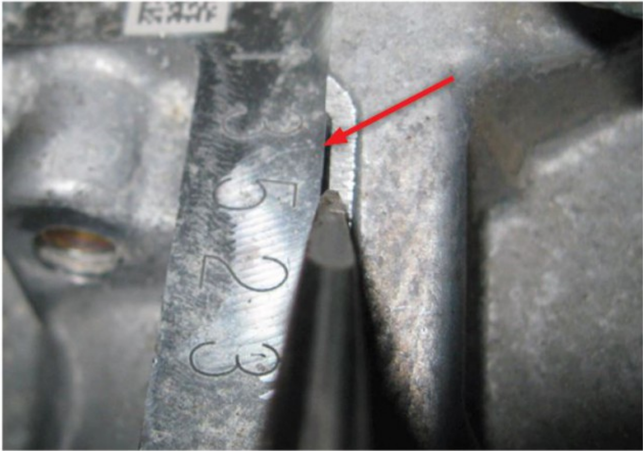
separating the transmission (CVT) from the engine pry relief
