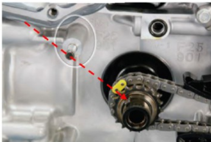
indicator link with the timing mark on the crankshaft sprocket
