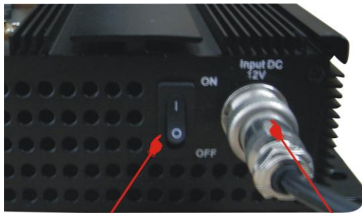
主电源开关 (ON开机, OFF关机) The switch of system's 直流电源插孔 (DC 12V Power Jack) Main power supply
