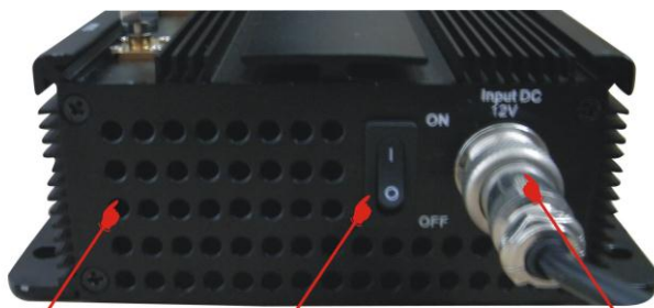
散热孔, 风扇内置 Cooling holes. 主电源开关 (ON开机, OFF关机) The switch of system's 直流电源插孔 (DC 12V Power Jack) Main power supply
