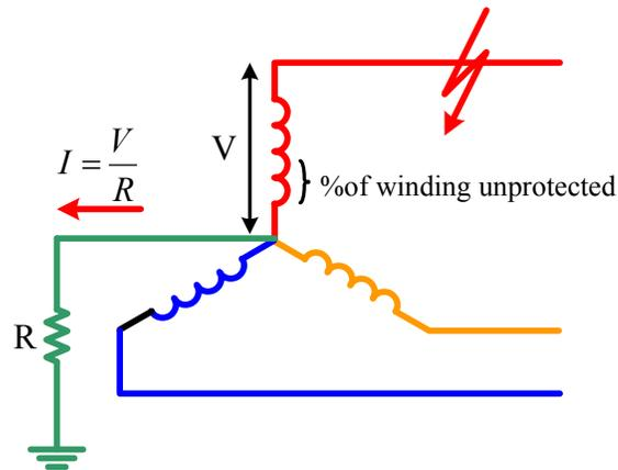
Assume R is the resistance in neutral connection to the earth and the fault current for line to ground fault is equal to full load current of the generator or transformer; the value of impedance to be inserted in neutral to earth connection is given by:  $R = \frac{V}{I}$ ,
