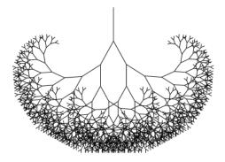
If the calls to save and restore were not there, the second recursive call to branch would end up with the position and rotation created by the first call. It wouldn't be connected to the current branch but rather to the innermost, rightmost branch drawn by the first call. The resulting shape might also be interesting, but it is definitely not a tree.
