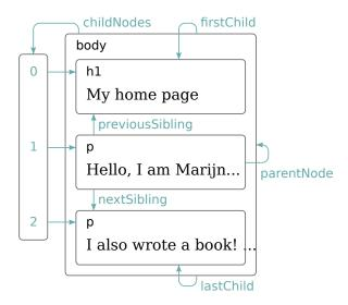
Although the diagram shows only one link of each type, every node has a parentNode property that points to its containing node. Likewise, every element node (node type 1) has a childNodes property that points to an array-like object holding its children.
