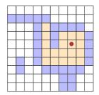
The flood fill does not leak through diagonal gaps and does not touch pixels that are not reachable, even if they have the same color as the target pixel.
