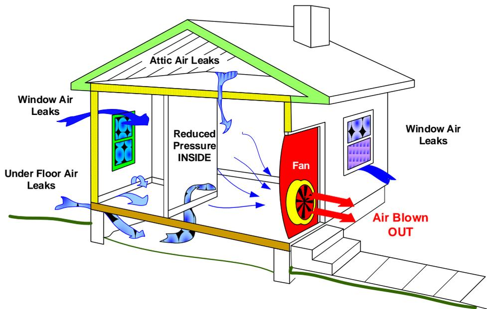
The **Air Tightness Test** involves the use of a large fan (Blower Door) installed in a temporary frame in one of the buildings doorways and closing all other external windows and doors. Any 'intentional' ventilation openings are closed or temporarily sealed during the test. (*Chimney, boiler flue, window vents, cooker hood and ventilation systems etc.*) All internal doors are kept open while the test is run.
