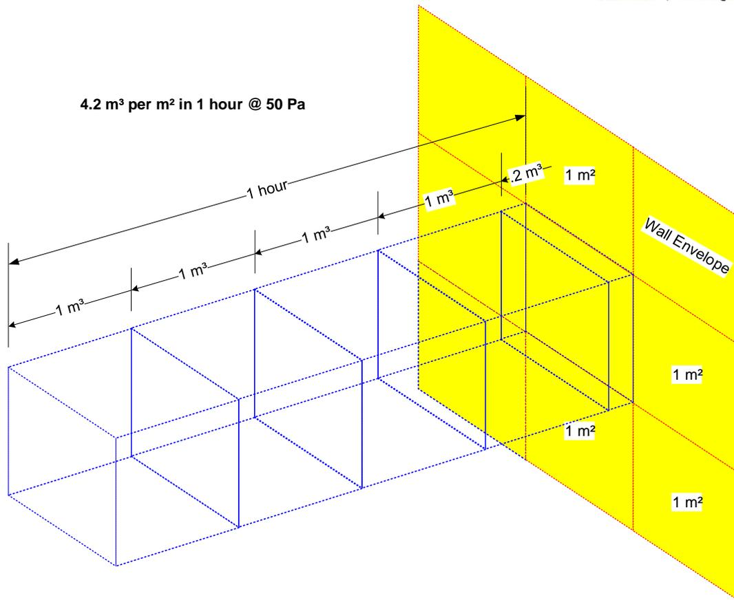
Sketch - Illustrating  $4.2\text{m}^3/\text{m}^2/\text{hr}@50\text{Pa}$
