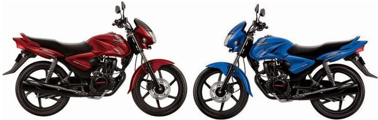
**Honda CB Shine** is the best two-wheeler of India in current times. It is an ideal combination of good power, high mileage and style. The **CB Shine** is propelled by a 124cc single cylinder air-cooled engine which has a peak power figure of 10.12 bhp at 7500 rpm and a peak torque of 10.54 Nm at 5500 rpm. The engine is linked to a four-speed gearbox and the fuel efficiency is rated at 65 kmpl.
