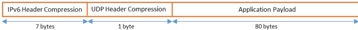
Figure 13. Application Payload in the Case of Multi-hop Transmission with IPv6 Header Compression
