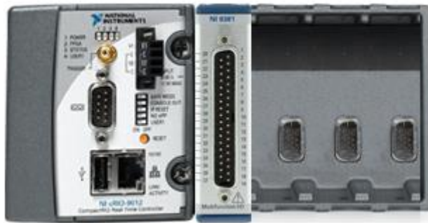
Figure 32. System Control Chassis, controller, and I/O Module
