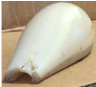
Figure 42. 3D Model (Cracks happened after testing)
