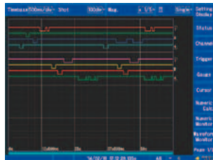
• Multi-channel timing measurement using logic waveform measurement
