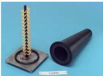
The *helix, or helical antenna* is quite a special case of antenna because it features circular polarization and looks pretty funny. Helix antennas have great bandwidth, are easy to construct and offer good noise immunity and immunity to phase cancellations due to the circular polarization.
