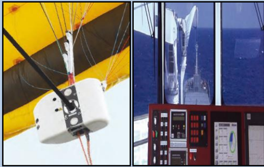
Fig 3 : Control pod and control unit system
