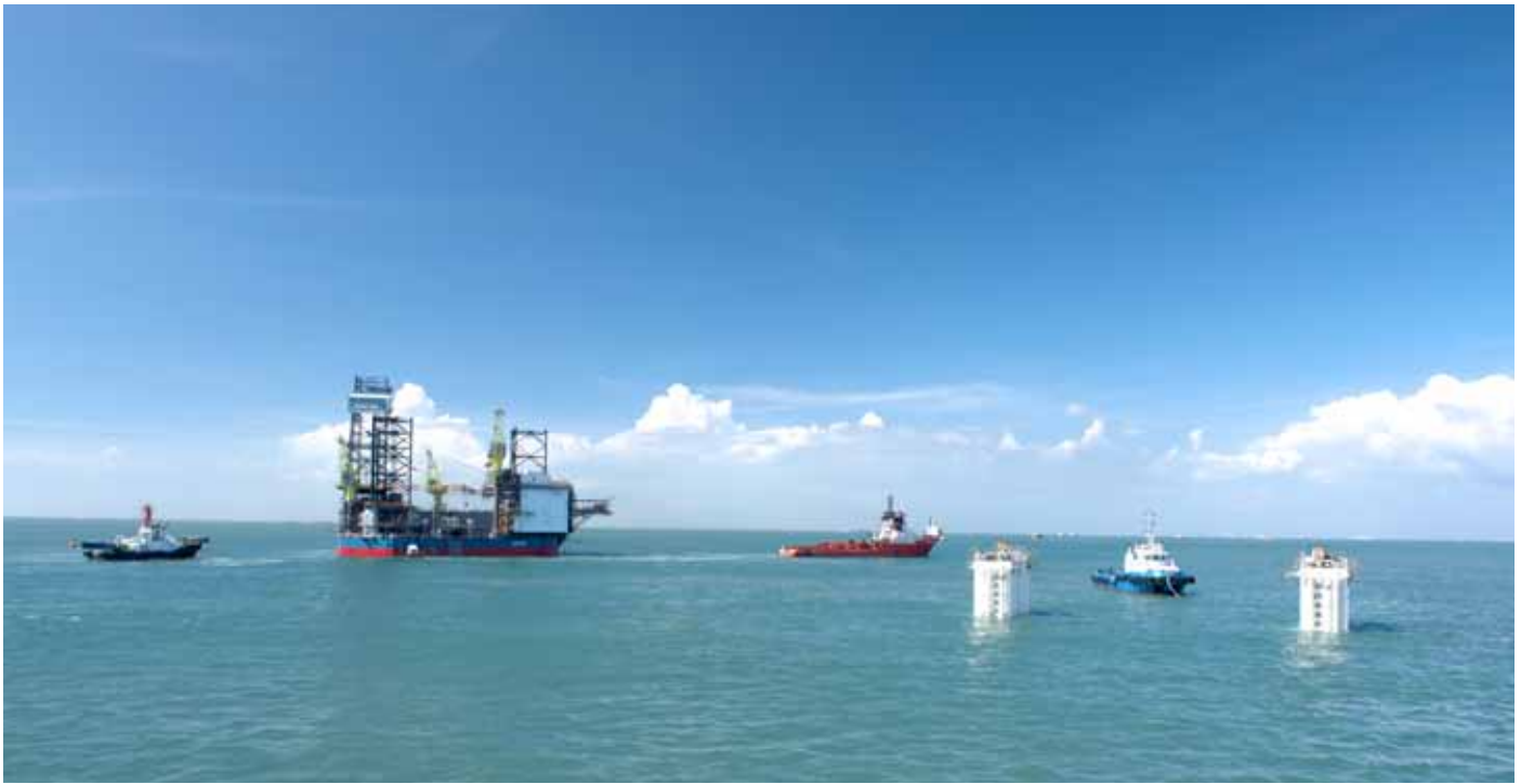
Float off completed, TAM DAO 5 handed over to harbour tugs
