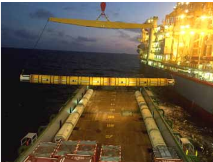
4,100DWT DP2 PSV POSH Skua loading up on risers at offshore Luanda, Angola
