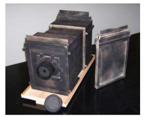
surfaces with a matte black spray. The camera was disassembled and painted in many very light coatings so as to avoid obstruction of the moving parts. The camera was finally fully completed and ready for use. The structure itself was strikingly beautiful in a sculptural sense. The completion of the camera alone was enough of a rewarding experience to satisfy me completely; however, the second half of the project, the task of actually making exposures, was only just ready to begin.
