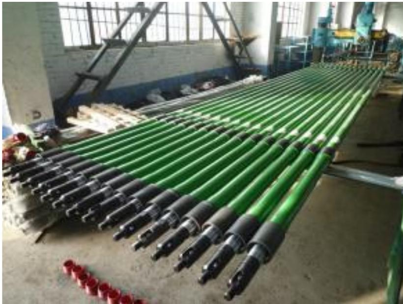
When the piston down, the liquid in pump is compressed followed by its higher pressure which equal to the pressure of liquid column in the annular space. Fixed valve will closed by its gravity. When the piston down continuously, the pressure in pump continues to rise. Until it is higher than column pressure, will the liquid lock traveling valve and enter the oil pump.
