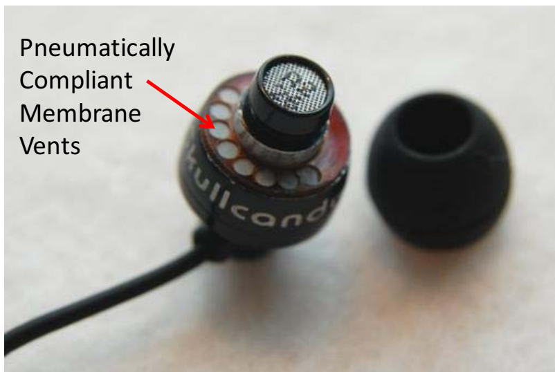
FIGURE 5: Modified Ear Tip with pneumatically compliant membrane vents (PCMV's)
