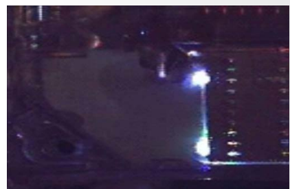
When Sufficiently Cool, Charged Particles Recombine And The Fault Current Is Stopped Quickly & Safely
