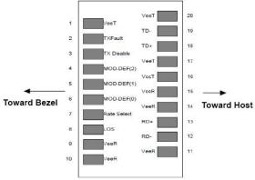
**Pinout of Connector Block on Host Board**
