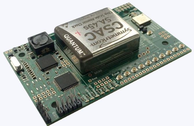
Alternative credit card-sized unit for internal server installation.
