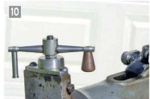
Crank handle installed on the feed screw.
