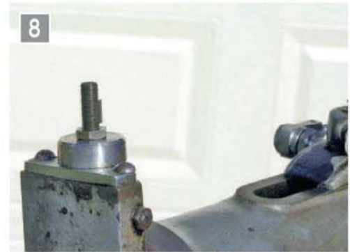
Collar and nut on the tool post.
