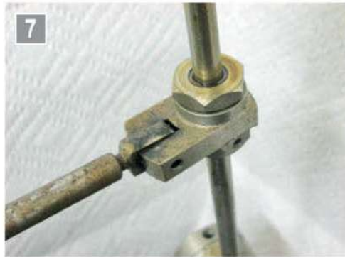
Ram rod - swing arm connection.
