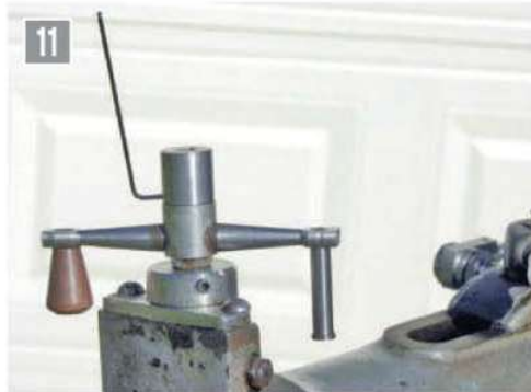
Quarter inch socket adapter installed on the feed screw.
