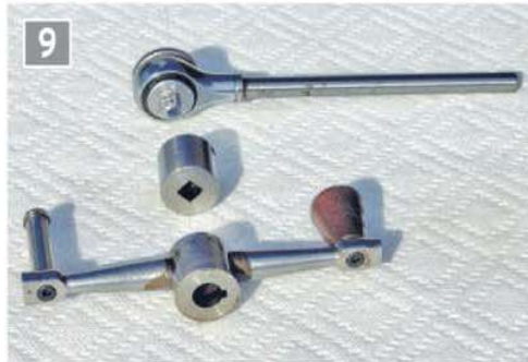
Upper tool post components.
