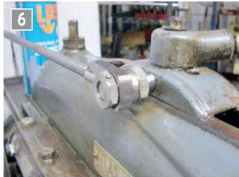
Ram rod - hinge pin connection.
