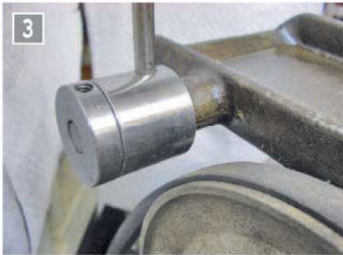
Swing arm boss and retaining ring.
