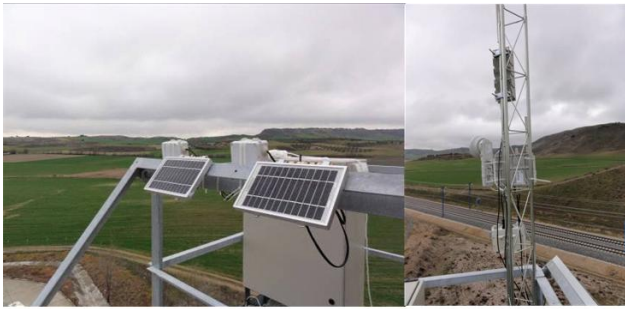
Figure 2. Autonomous nodes located in a post at 15 m of altitude next to the railway infrastructure
