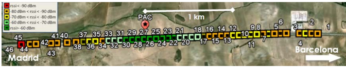
Figure 1. Location of measurements along the railway infrastructure
