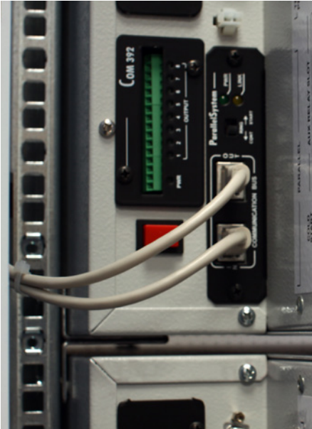
Parallel configuration and programmable relay contacts board
