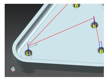
operations. When doing the top face of the bracket in denford, the wholes are drilled again, where as in Nx you can simply specify them not to get cut. The holes are a good example of this. Using denford I was not able to specify the holes did not need to be cut when working on the top face of the bracket.
