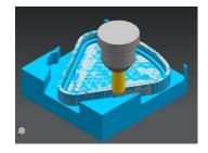
Now the streamline method can be used to cut the rounds using a 6mm ball end cutter and Mill-Finish. Originally this did not give a good finish but after adding steps before the operations it works well. The last thing for the back is to use a Z-profile with standard 6mm carbide drill to drill the holes. This operation makes the cutter drill down into the hole and then moves in circular motion to cut the hole out.
