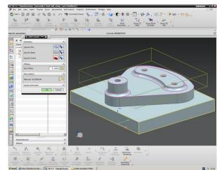
semi-Mill was selected instead of Mill-Rough-finish. This removed more material. I then used another cavity mill with semi finish to remove left over material. To cut the rounds contour area was used but problems with the cutter colliding with part where the raised hole is. Switching to a 10mm ball end still collided. End mill did not collide but did not leave a smooth finish at all.
