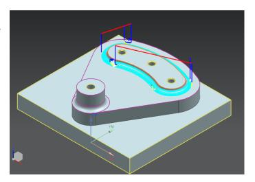
For both operations I used the 6mm ball nose which collided with the extrusion even after changing the tool to an 8mm and then 10mm. I made my own tool because none where big enough in the tool library. The cutter has 8mm diameter with a 25mm flute length. This was big enough not to collide with the hole.
