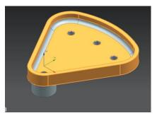
same cutter as the pervious operation which is the 20mm end mill tool. The finish was also changed from Mill-semi-finish to mill-finish. Now that outside has been cut away the Z-level was not used for the rounds but to go over the cuts made around the outside of the bracket and on the inside above the rounds. This is an operation that was missed out when first attempted.
