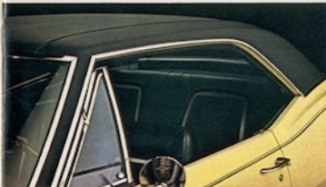
Bright drip gutter molding for sport coupes.
