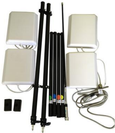
Directional Antennas with Frame 7dBi : 800-965MHz 9 dBi: 1710-2500MHz Size: 200 x 180 x 45mm
