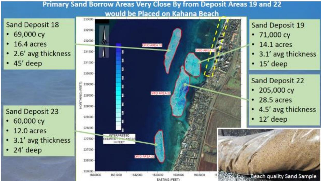
**Figure 3. Four major Sand Deposits Surveyed.** Beach quality sand borrowed from nearby offshore deposit areas can be dredged up on shore to the Kahana Beach along each of the condos in a continuous manner, resulting in a restored beach. The sand has been found and this sand survey has made regional beach nourishment a realistic and cost-effective option.
