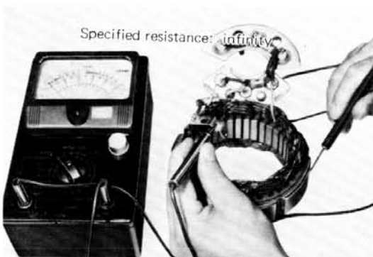
Fig. 5-15 Testing Stator Coil for Insulation
