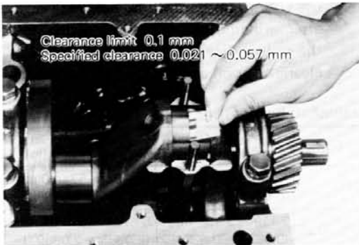
Fig. 1-46 Measuring Oil Clearance
