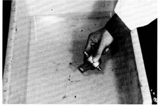
Fig. 2-38 Fuel Filter Inspection
