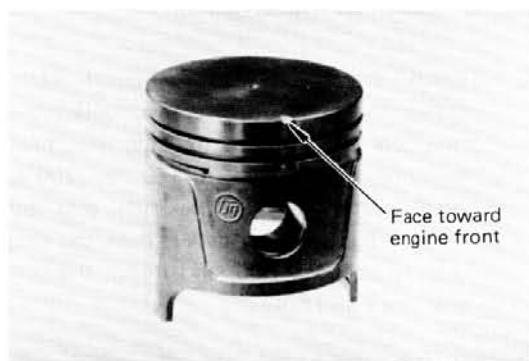
Fig. 1-59 Piston Front Mark
