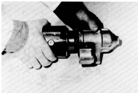
Fig. 6-7 Yoke and Armature Removal
