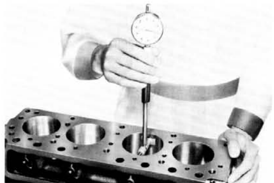
Fig. 1-34 Measuring Cylinder Bore
