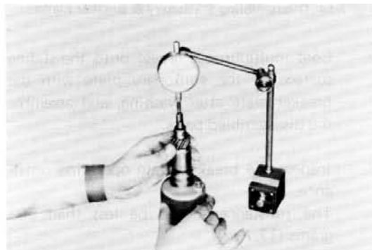
Fig. 7-12 Checking Thrust Clearance
