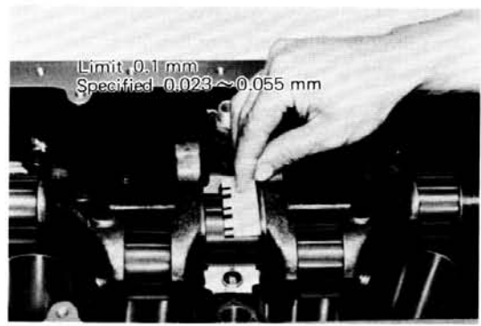
Fig. 1-49 Measuring Oil Clearance
