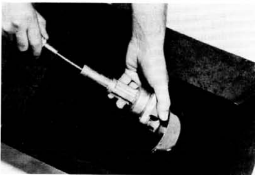
Fig. 3-9 Oil Pump Test
