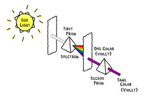
He adjusted the prism so that only the violet-colored light passed through the tiny slit in the screen. He placed a second prism on the other side of the screen and allowed the violet light to pass through that prism also. The light coming through the second prism was still violet. The
