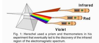
The temperatures of the different colors varied slightly, but, most surprisingly, the hottest temperature was just *beyond* the red band. This was the first indication of invisible light and led to the discovery of **infrared (IR) light**. If you've studied Latin, you may remember that "infra" means "below" or "lower than." Infrared light was thought of as "below" the red color on the light spectrum.
