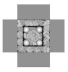
Separate the products from the walls of the container with a minimum of 2 inches (5.08 cm) of recommended materials.
